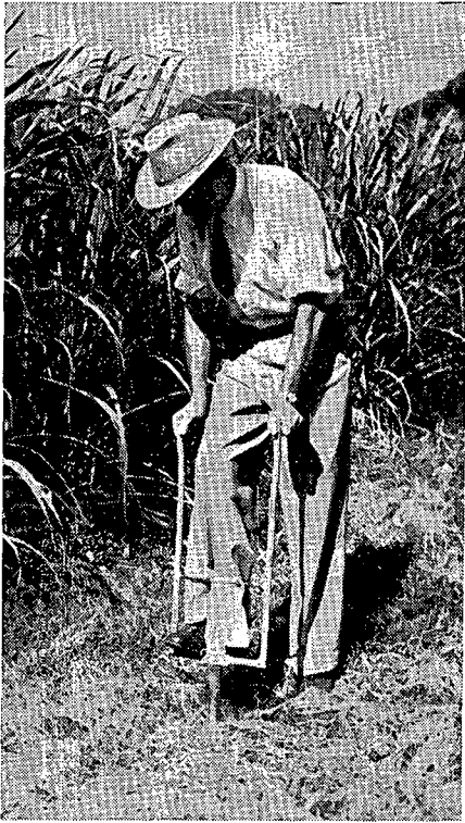
Fig. 3—Thrusting and twisting the sampler into the soil
