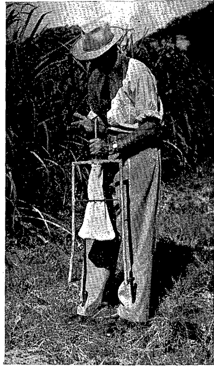
Fig. 4—Removing the soil core by thumping the tube
