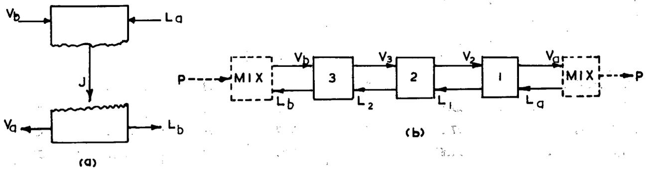
FIG. 6 OVERALL BALANCES IN LEACHING SYSTEM
