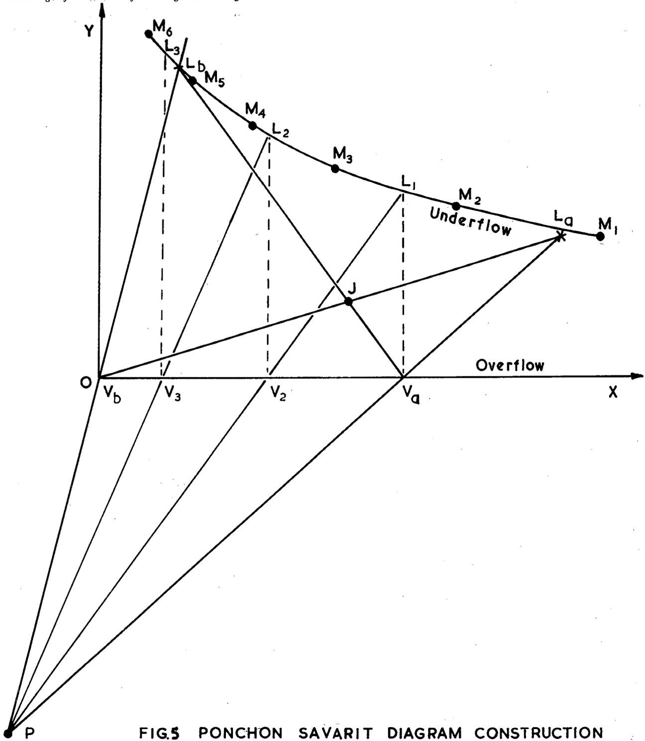
FIG. 5 PONCHON SAVARIT DIAGRAM CONSTRUCTION
