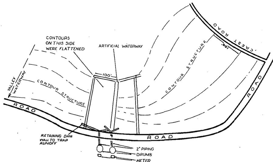
FIGURE 1: Layout of Field 37, Inyaninga Section.
