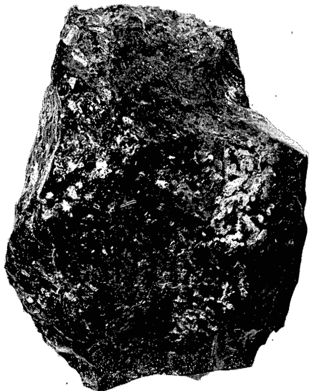
B. Vitrified deposit taken from boiler arch brickwork. 3" maximum horizontal dimension (thickness).
