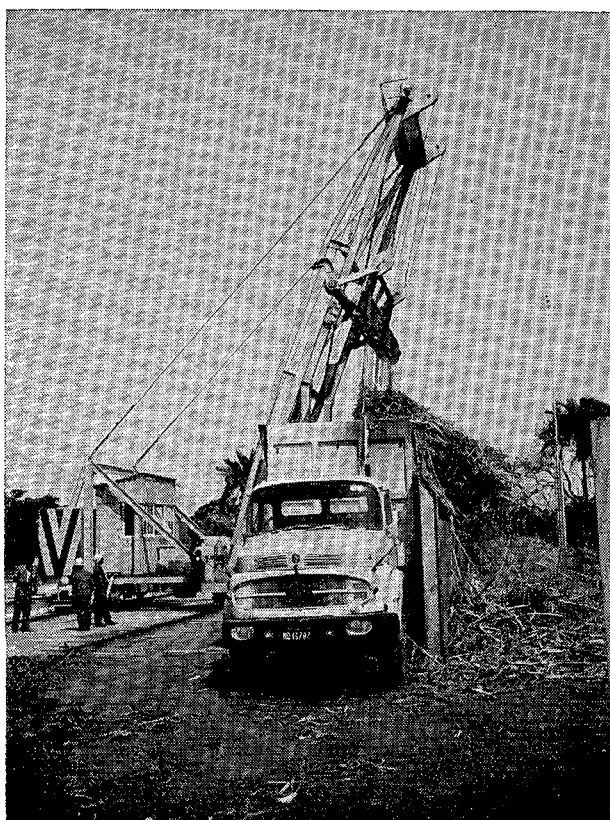
FIGURE 5 Hilo trailer being off-loaded and the "loose" or "bulk" cane being spilled on to the mill yard floor.
