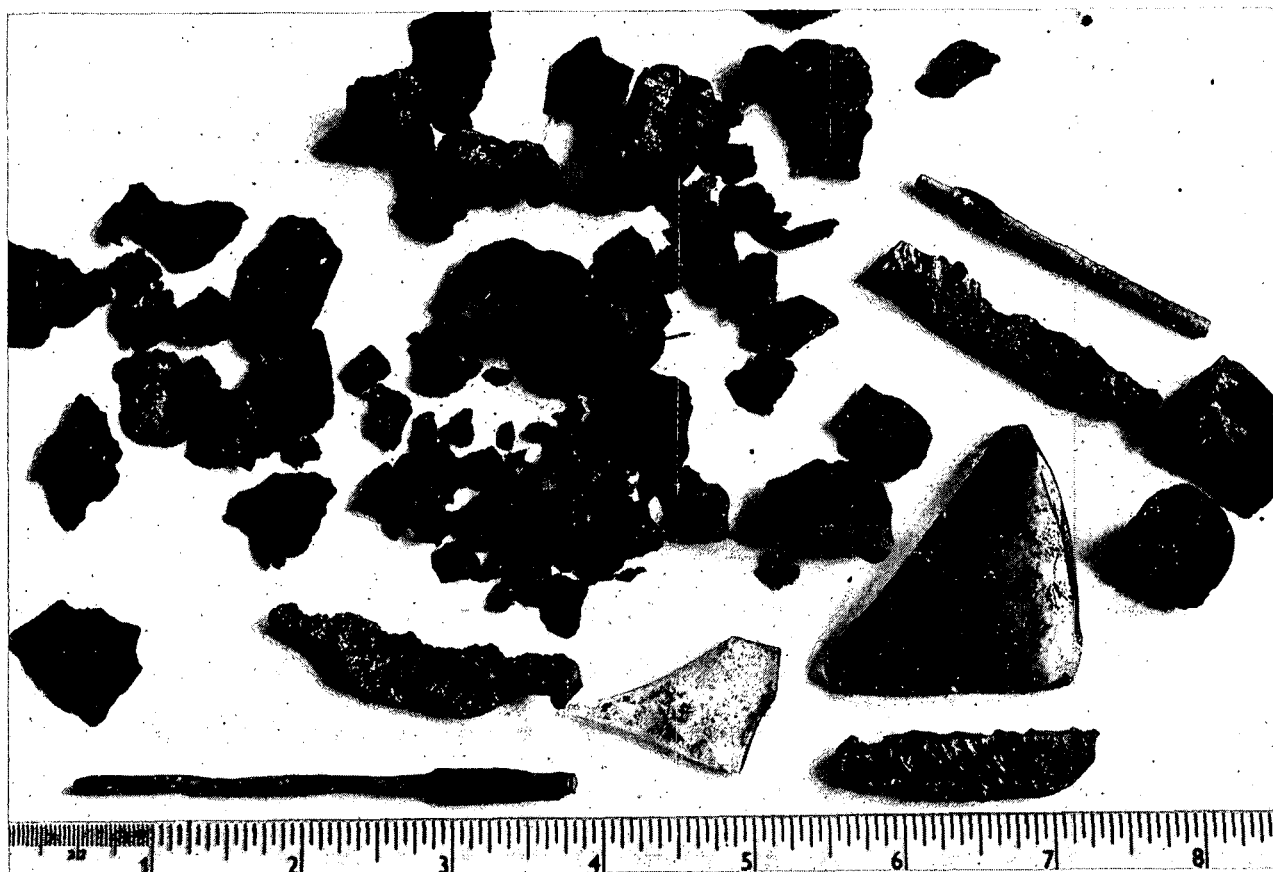
FIGURE 8 Typical debris removed from continuous centrifugals. (scale: in inches)
