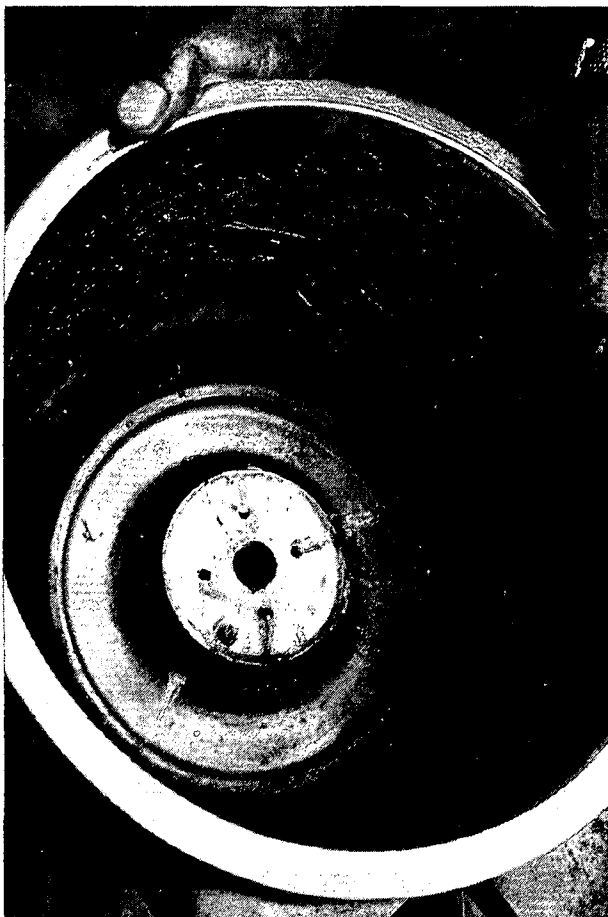
FIGURE 7 Scaling on the inside of an accelerating cone.
