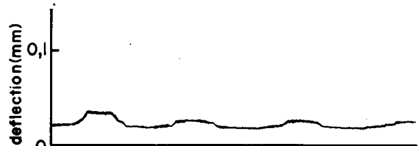
FIGURE 6 Recording of torque under no load conditions.
