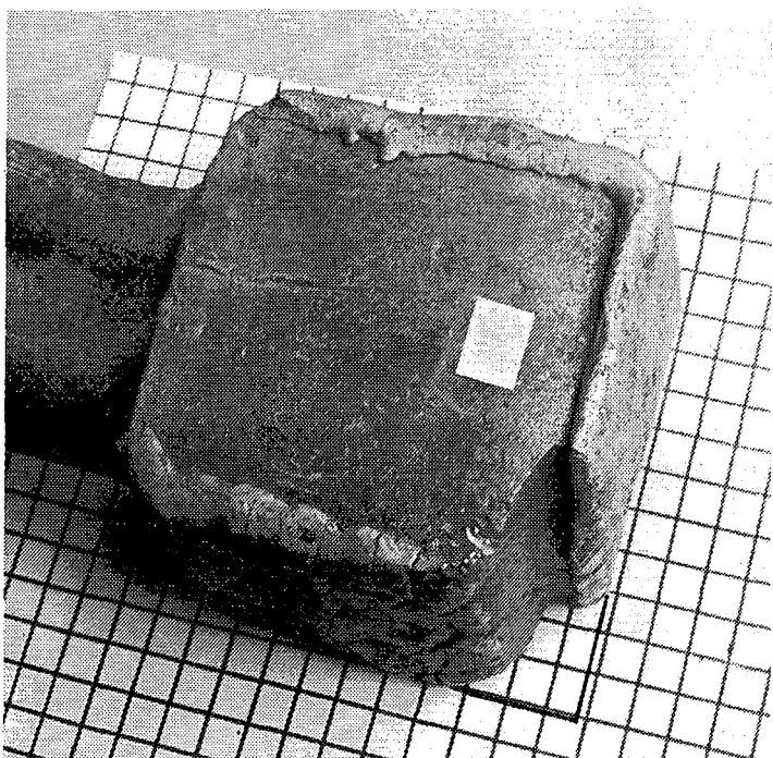
FIGURE 4 Worn but square shredding edge.
