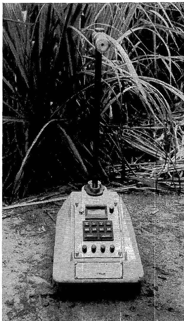
FIGURE 1 Troxler nuclear density and moisture gauge.
