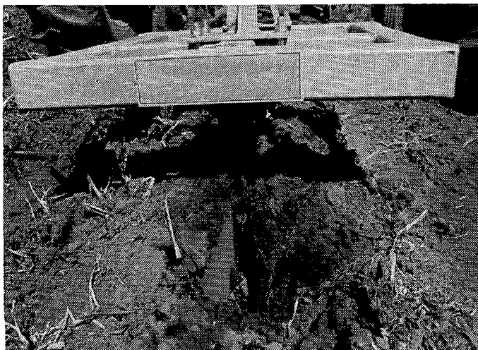
FIGURE 1 The implement used for vertical mulching.
