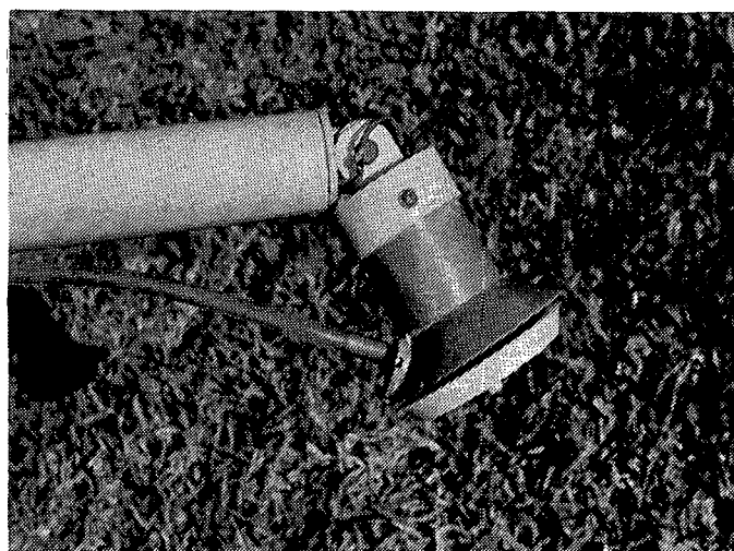
FIGURE 1 Modified spinning disc controlled droplet and applicator.
