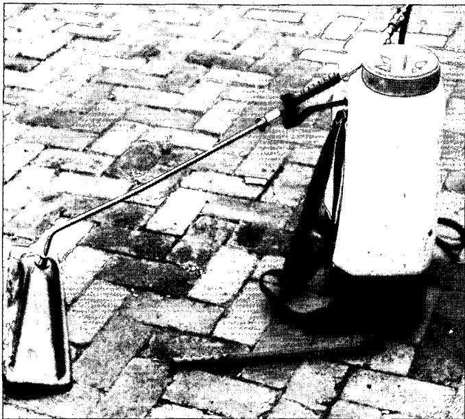
FIGURE 2 Conical shield fitted to the lance of a CP3 knapsack sprayer.
