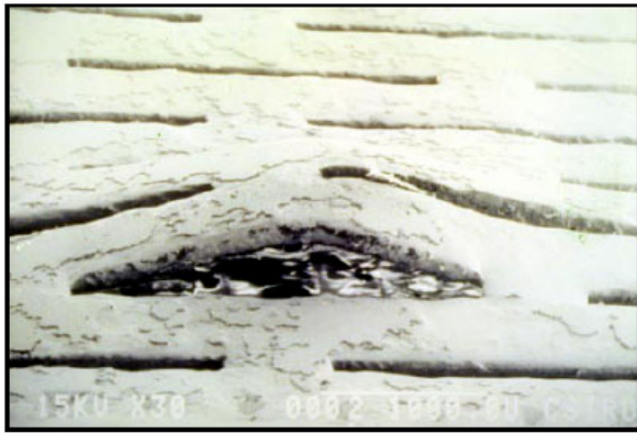
Figure 1 This illustrates the deformation and slot enlargement that occurs in chrome nickel screens. 1000 microns |————|
