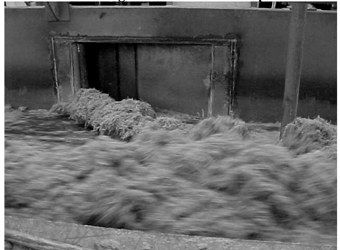
Bagasse being diverted into a feed chute
