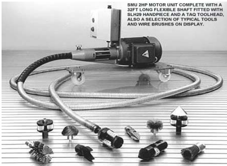
Figure 1. An example of the equipment used in mechanical cleaning of evaporators in a sugar factory.
