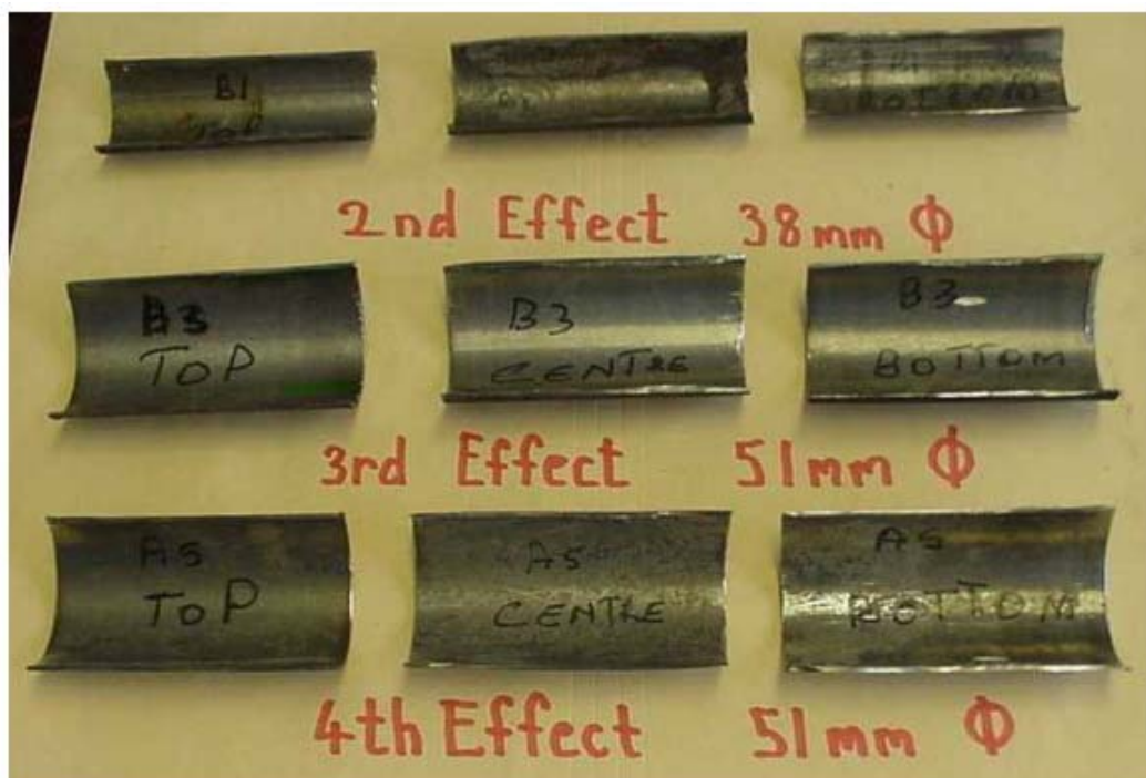
Figure 5. Inside sections of cleaned evaporator tubes.
