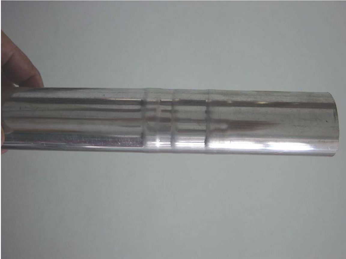
Figure 3. Tube damage caused by the cleaning tool being run at high speed under dry conditions.
