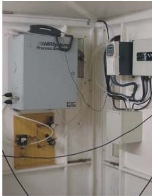
Figure 3. Inside the NIR cabin at Maidstone, showing the NIR Systems 6500 process spectrometer (mounted on rubber isolators). The PID controller for the discharge rolls is shown on the right.
