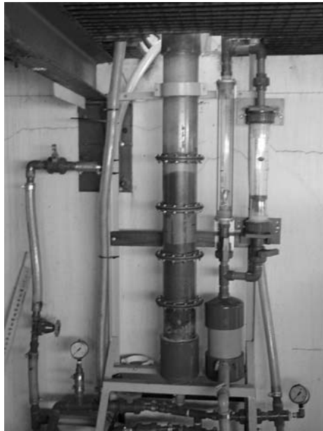
Figure 1. The DBF pilot rig.
