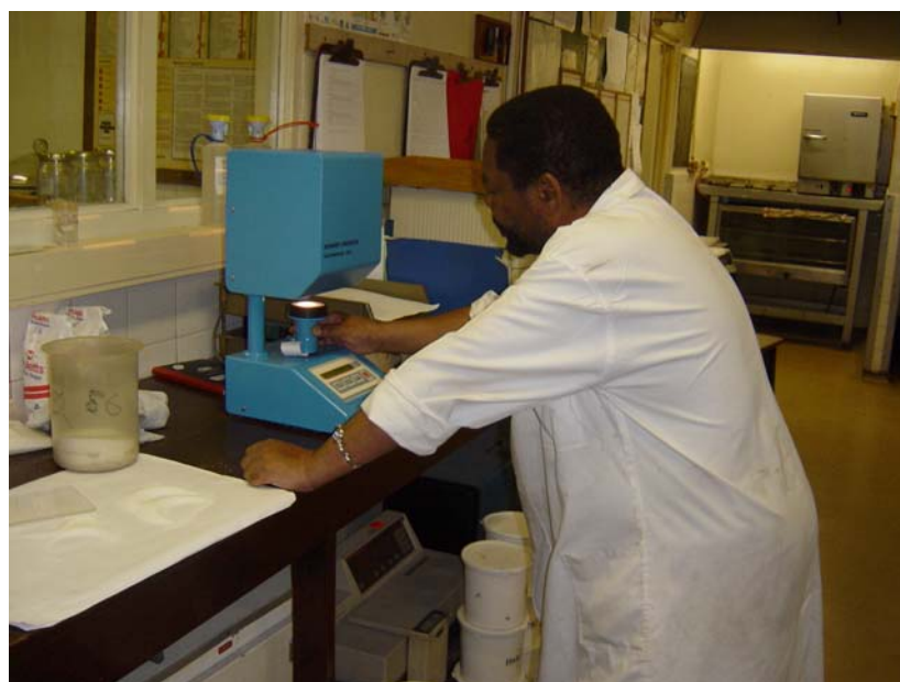
Figure 2. Hulett's refinery analyst using the Saccharoflex 2000 instrument to read the reflectance of a refined sugar sample.
