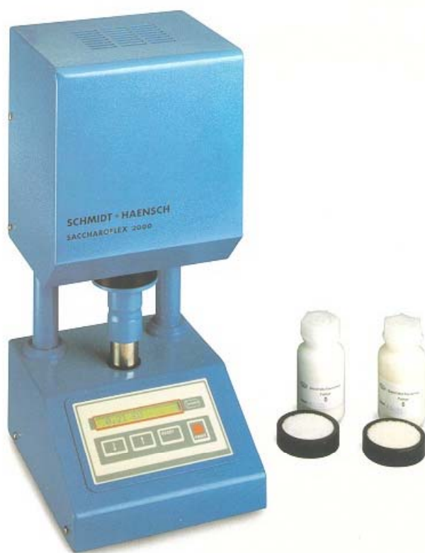
Figure 1. The Saccharoflex 2000 colour measuring system.
