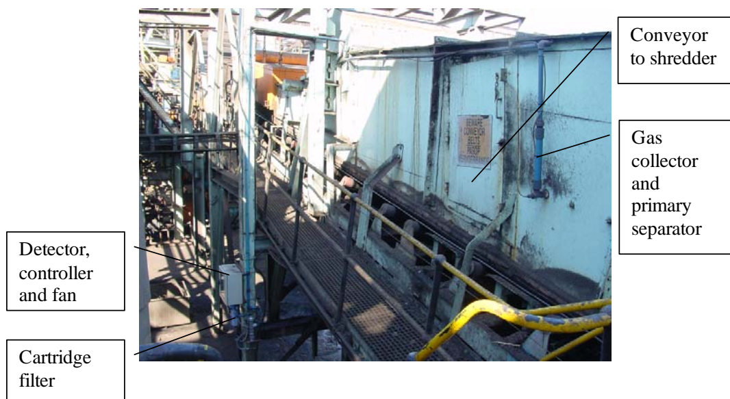
Figure 2. Ethanol detector mounted just after knives.
