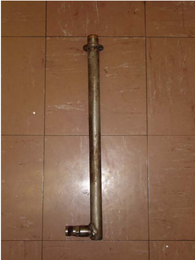
Figure 1. Spray bar with single fan spray nozzle.
