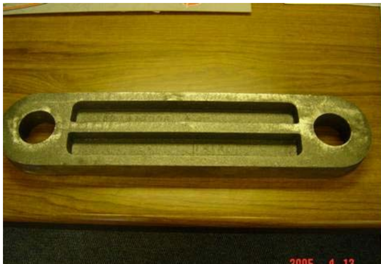
Figure 3. Experimental side link with added centre stiffener.
