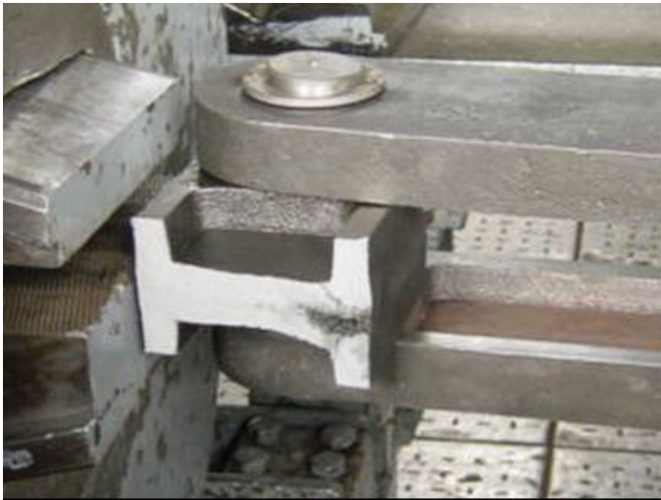
Figure 12. Failed new link 1 sample.
