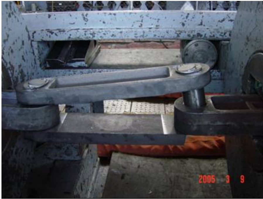
Figure 18. Failed new link 3 sample.
