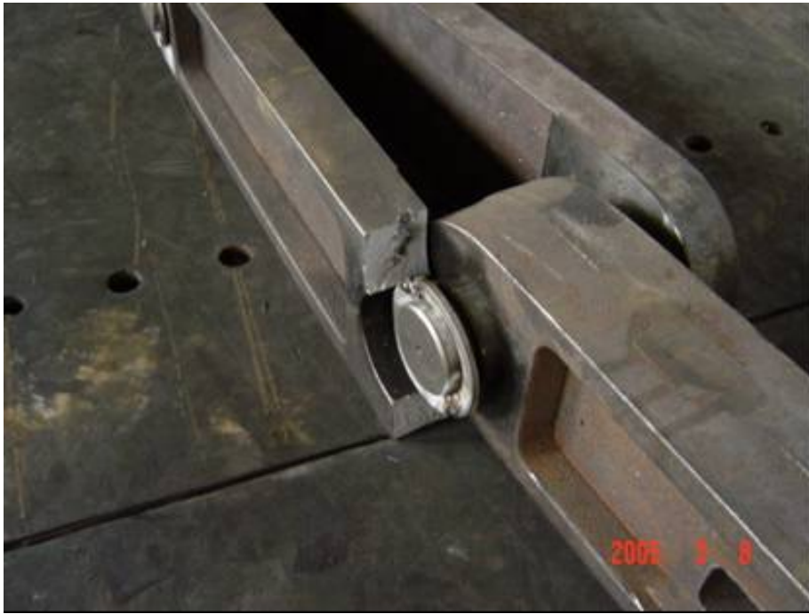
Figure 16. Failed defective new link 2 sample.
