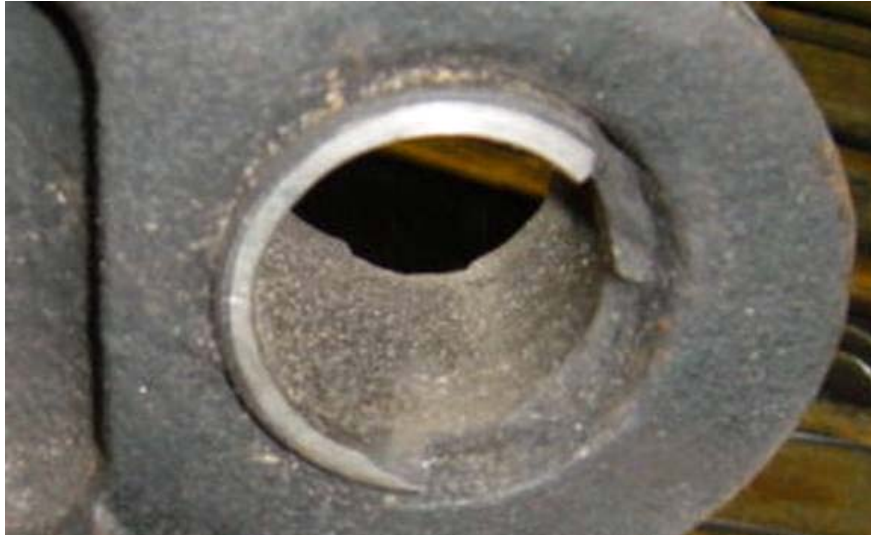
Figure 2. Worn Ausrex inner link.
