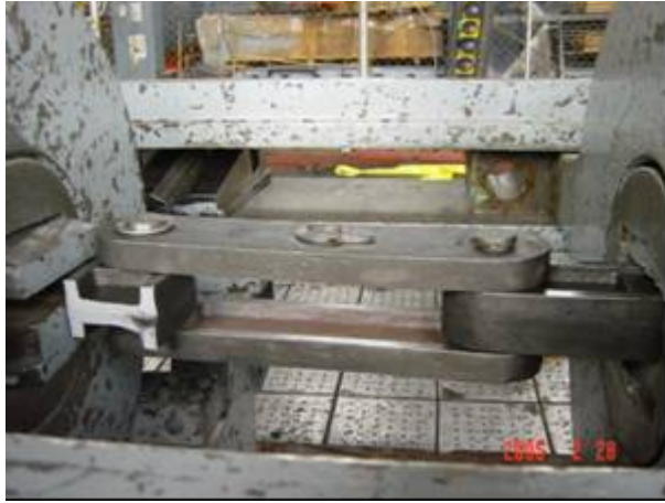
Figure 7. Failed ADI chain with defect.
