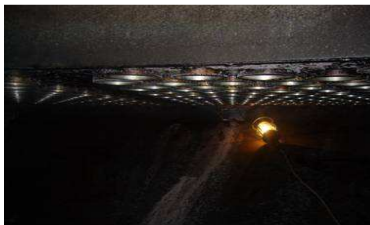
Figure 10. White trail of syrup/massecuite on AK batch pan 1 saucer.
