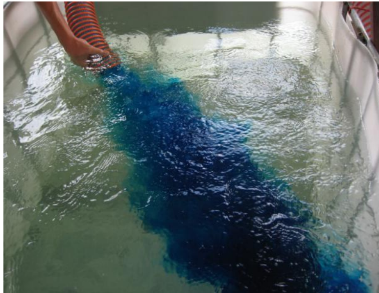
Figure 2. Tracer injection into a water tank (pipe diameter 8 cm, flowrate 23 m 3 /h).
