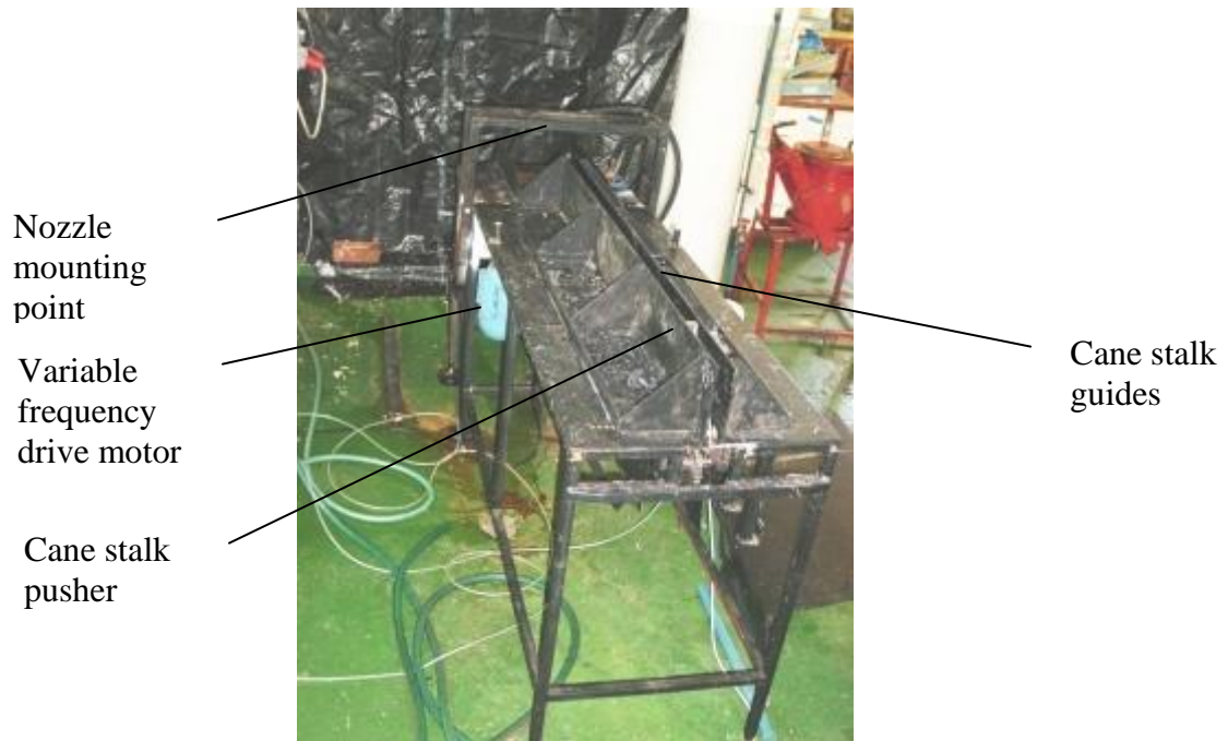
Figure 3. General layout of first Prepex apparatus.
