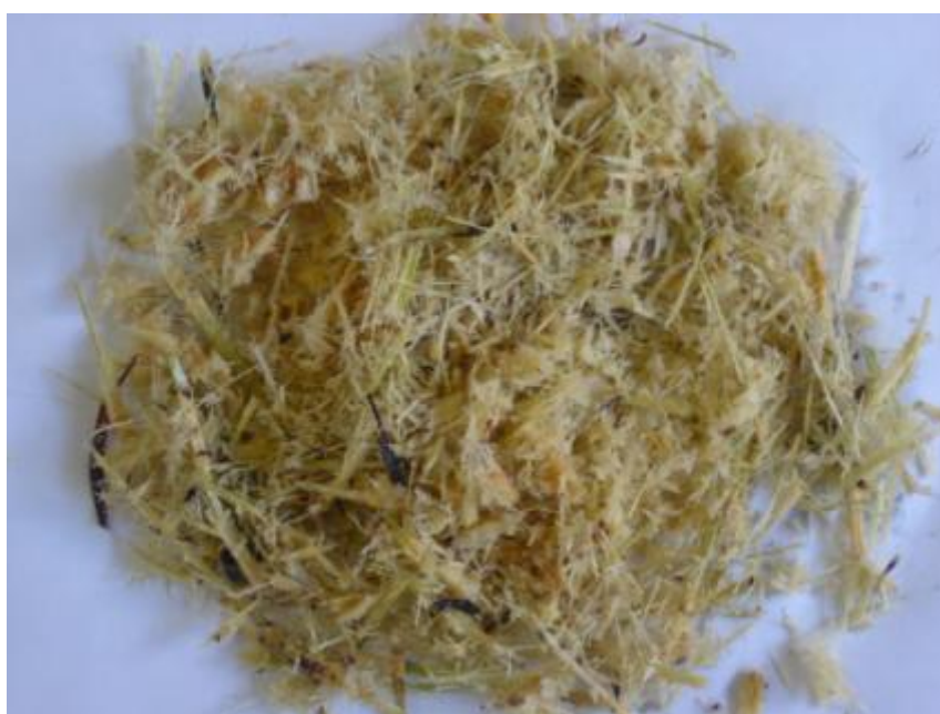
Figure 6. A sample of Prepex-prepared cane.
