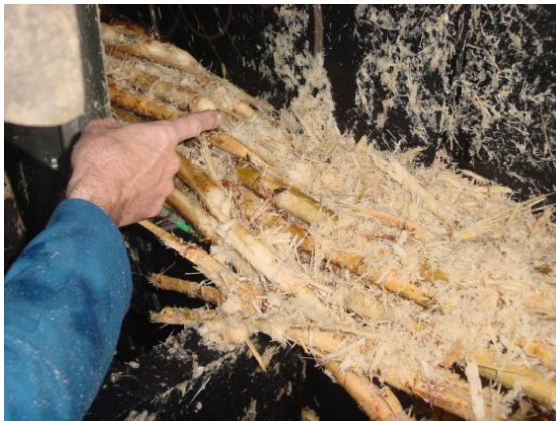
Figure 5. Stopped test indicating how cane is shredded in layers.
