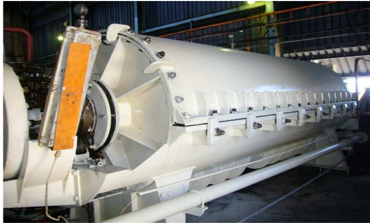
Figure 2. Rotary pressure leaf filter at Pongola.
