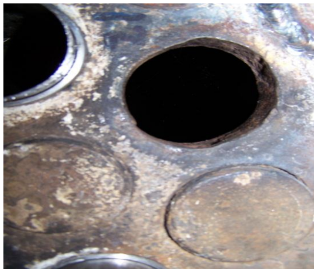
Figure 3. Tube sheet with distorted tube hole.
